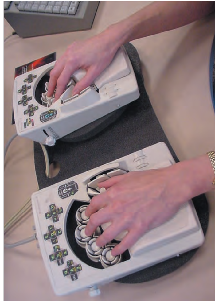
Ms Prine demonstrates the Datahand ergonomic keyboard. With four modes, shifted by the thumbs, hand movement is no longer required to perform keyboard work. A boon for repetitive strain injury sufferers.
