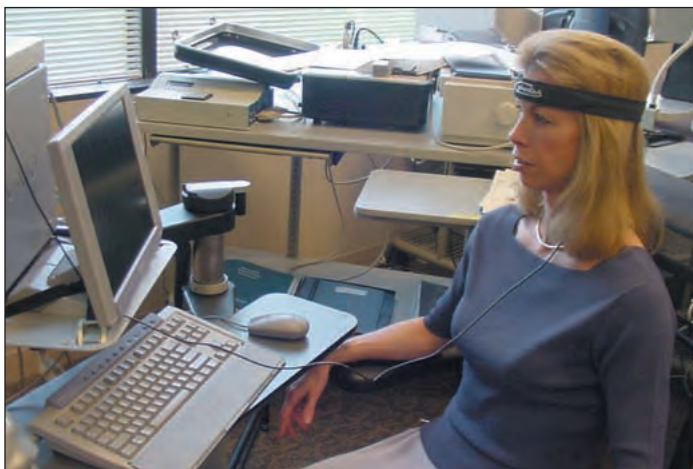
Martha Prine demonstrates Cyberlink, from Actuated Technologies. This enables the wearer to direct a computer mouse with a headband.
