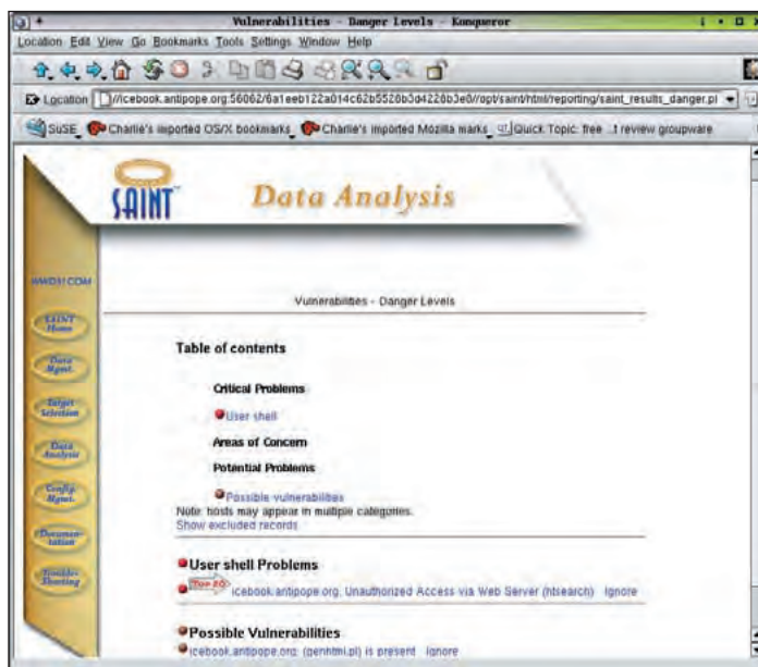
Saint uses a 100% web-based interface. The data analysis page shows a vulnerability, revealed in the results of a SAINT -scan of a local machine.
